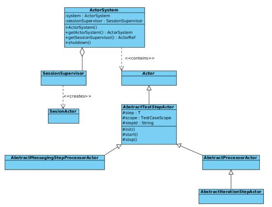
Figure 10-14: Class Diagram of the Actor System Based on Akka
